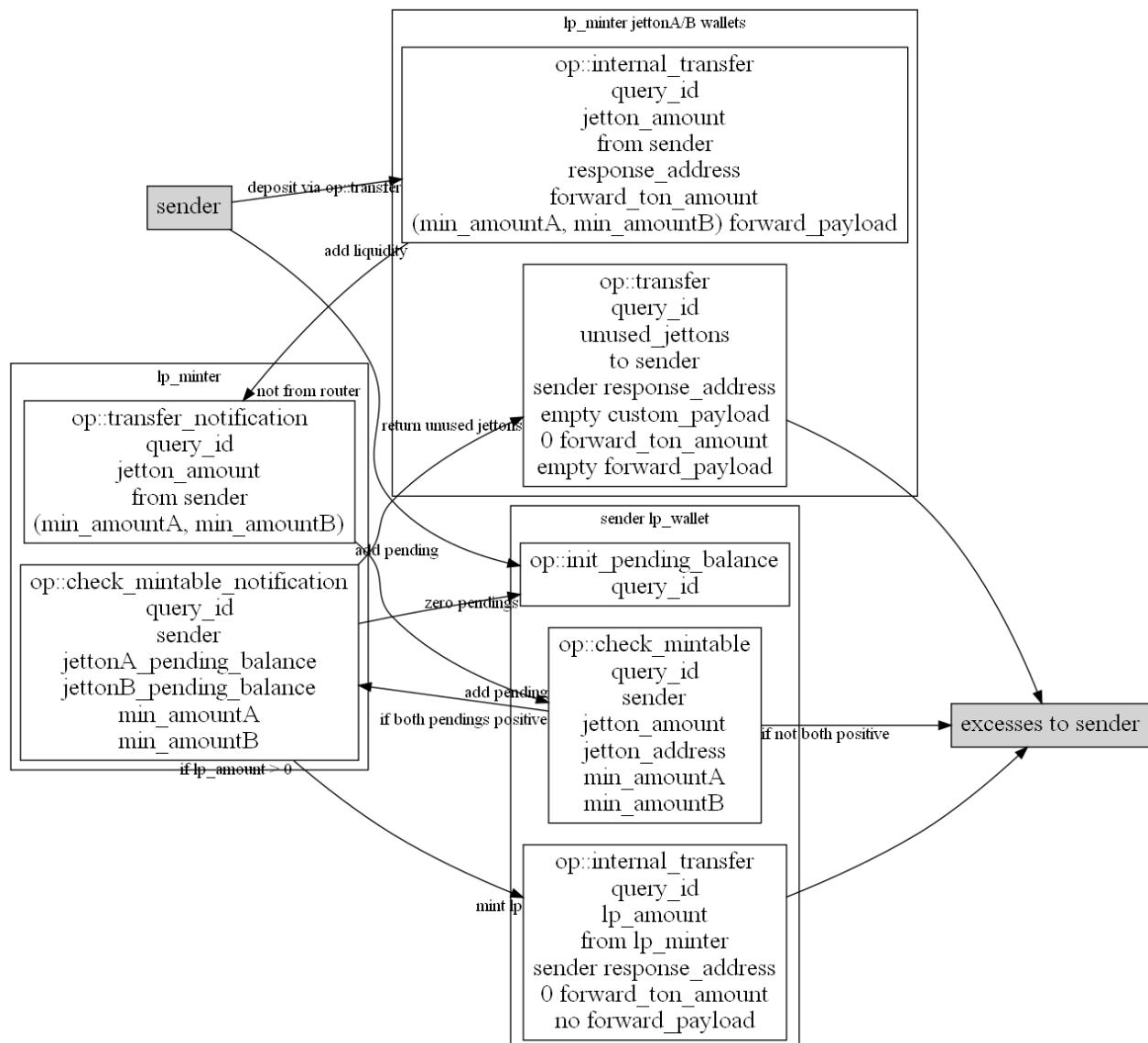
Handling of `op::check_mintable_notification` at `lp-minter` works this way:
